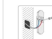
Remove the existing doorbell A from the wall and disconnect
