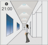
The light switches on at 100% when there is movement detected. The light dims to stand-by level after the hold-time.
