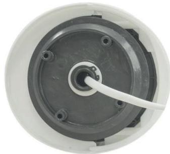
**IMPORTANT:** Make sure that the power cord passes through the slot on the rear half of the base.
