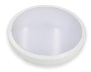
This fitting is a 24W LED bulkhead light fitting ideal for outdoor wall lighting. It has an IP65 rating (it is waterproof) and offers a 4000K light. With a 110mm projection and approx. 280mm diameter, this bulkhead has a poly carbonate base in white, a gloss white trim ring, and an opal diffuser.
